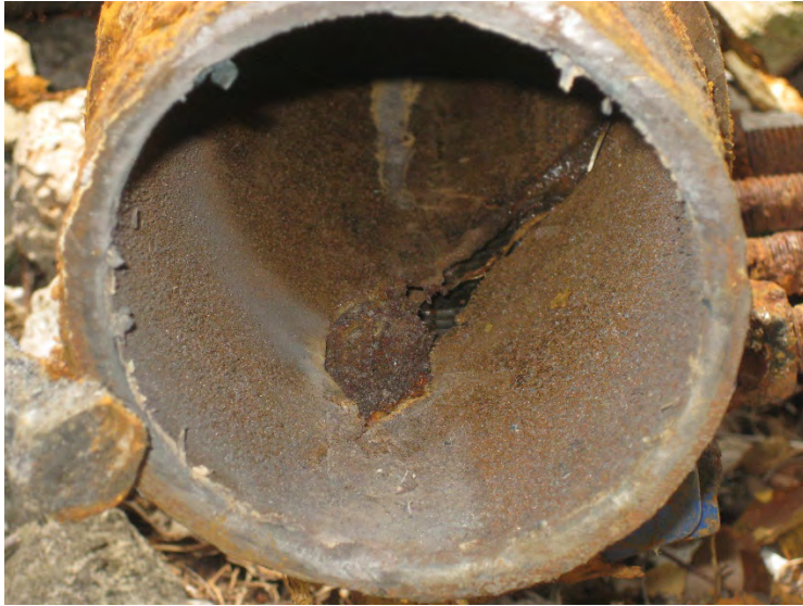
Figure 1: Piping removed from wet well with through-pipe corrosion
